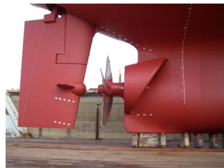
Figure 1.19 SURF-BULB (Courtesy of Japan Marine United Corporation)
