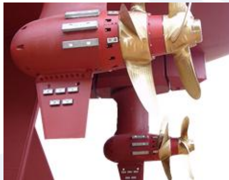
Figure 1.17 Contra-rotating Propeller (Courtesy of Nakashima Propeller Co., Ltd.)
